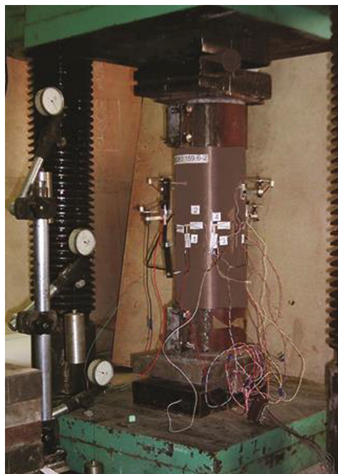
Fig. 1. General view of the sample during the eccentrical compression test
