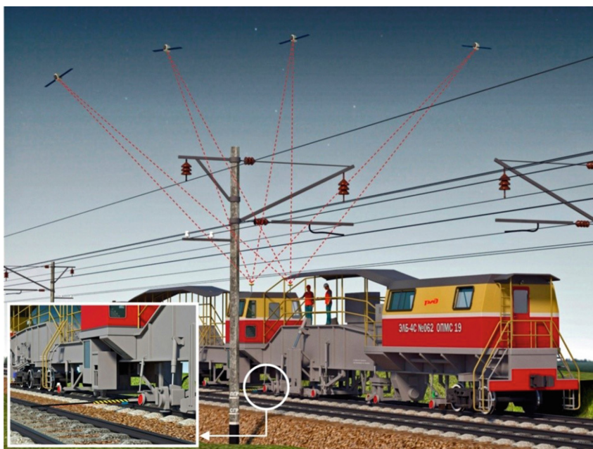
Fig. 1. Overview of an electrical ballast vibrator equipped with ACS-3D
