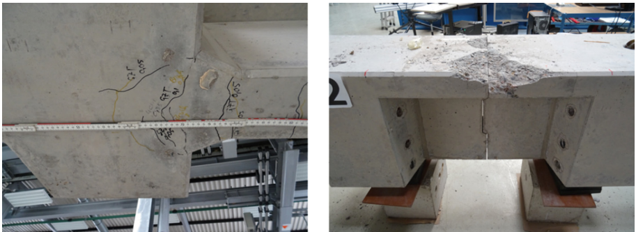
Fig. 7. Failed specimen, left: cracks at bottom side, right: failed concrete compression zone.
