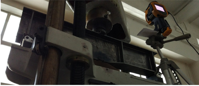
Fig. 2. The process of dynamic testing of the beam on the GRM-2a installation with a pulsator
