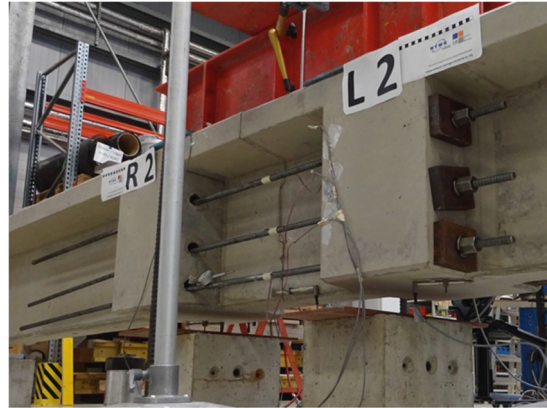
Fig. 2. Post-tensioning of the connection between the two precast elements.
